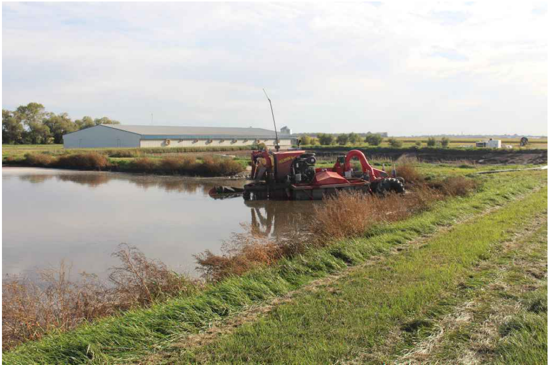
Nuhn boat agitator/pump in secondary at second strategy
