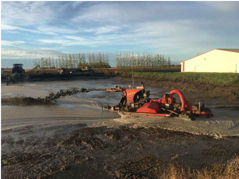
Nuhn boat agitator assisting in agitating concentrated primary cell at third strategy
