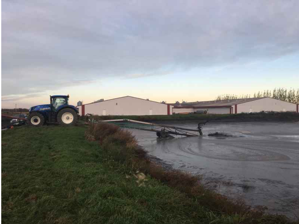
Tractor with Houle agitator/loading pump in concentrated primary cell at third strategy
